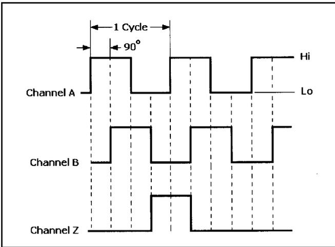
**Fig. 3** Channels A and B provide bidirectional position sensing. If channel A leads channel B, the direction is clockwise; if channel B leads channel A, the direction is counterclockwise. Channel Z provides a zero reference for determining the number of disk rotations.
