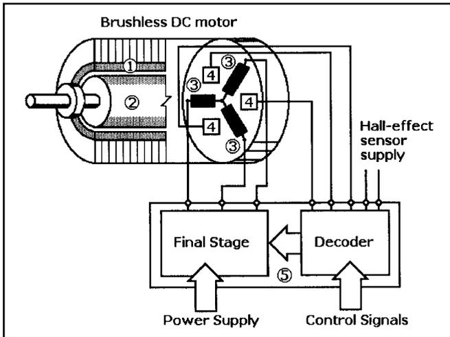
**Fig. 9** A magnetic sensor as a rotor position indicator: stationary brushless motor winding (1), permanent-magnet motor rotor (2), three-phase electronically commutated field (3), three magnetic sensors (4), and the electronic circuit board (5).
