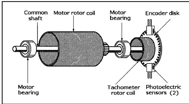
**Fig. 11** This coil-type DC motor obtains velocity feedback from a tachometer whose rotor coil is mounted on a common shaft and position feedback from a two-channel photoelectric encoder whose code disk is also mounted on the same shaft.
