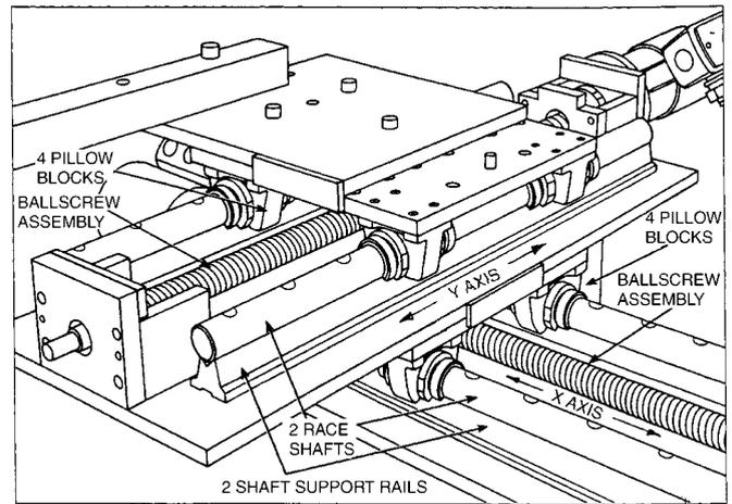
**Fig. 2** Microcomputer-Controlled X-Y Table: Catalog pillow blocks, rail guides, and ballscrew assemblies were installed in this rigid system that positions workpieces accurately for precise milling and drilling on a vertical milling machine. *Courtesy of Thomson Industries, Inc.*
