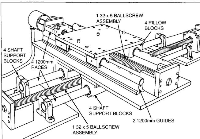
**Fig. 3** Pick and Place X-Y System: Catalog support and pillow blocks, ballscrew assemblies, races, and guides were in the assembly of this X-Y system that transfers workpieces between two separate machining stations. *Courtesy of Thomson Industries, Inc.*
