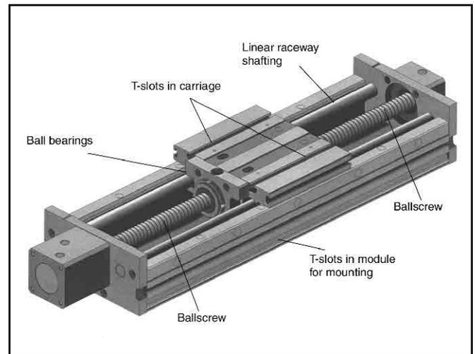
**Fig. 2** This commercial ballscrew-driven system also offers position accuracy of 0.025 mm per 300 mm with repeatability of  $\pm 0.005$  mm. It has T-slots in both its carriage and base mounting system, and is also designed to be continuously supported. *Courtesy of Thomson Industries, Inc.*
