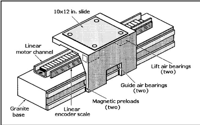
**Fig. 14** This single-axis linear guide for load positioning is supported by air bearings as it moves along a granite base.
