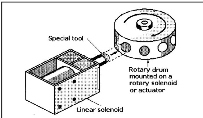
**Rotary Positioning:** A linear push-out solenoid is paired with a multi-station drum containing objects that are indexed by a linear solenoid or actuator. This arrangement would permit the automatic assembly of parts to those objects or the application of adhesives to them as the drum is indexed.
