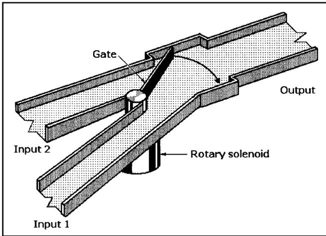
**Parts or Material Diversion:** This diverter arrangement consists of a rotary solenoid with a gate attached to its armature. The gate can swing to either of two alternate positions under pushbutton or automatic control to regulate the flow of parts or materials moving on belts or by gravity feed.
