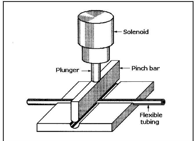
**Pinchoff of Flexible Tubing:** This push-out linear solenoid with an attached blade can control or pinch off liquid flowing in flexible tubing when energized by a remote operator. This arrangement can eliminate valves or other devices that could leak or admit contaminants. It can be used in medical, chemical, and scientific laboratories where fluid flow must be accurately regulated.
