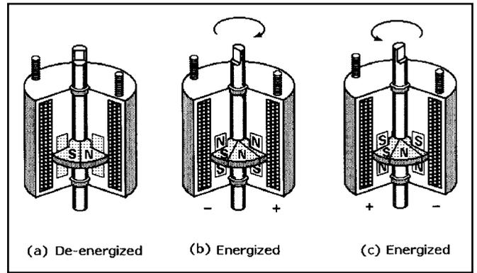
**Fig. 5** This bidirectional rotary actuator has a permanent magnet disk mounted on its armature that interacts with the solenoid poles. When the solenoid is deenergized (a), the armature seeks and holds a neutral position, but when the solenoid is energized, the armature rotates in the direction shown. If the input voltage is reversed, armature rotation is reversed (c).
