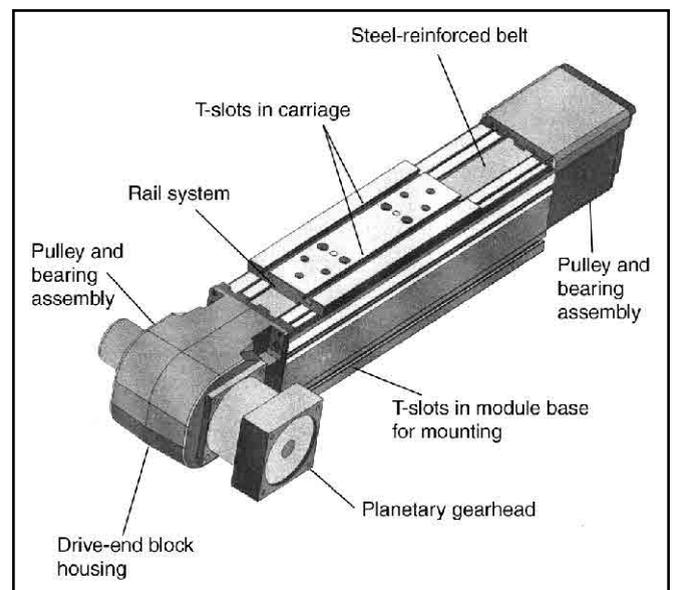
**Fig. 4** This modular single-axis belt-driven system is built more ruggedly for applications where a rigid, continuously supported module is required. With a planetary gearhead its mechanical characteristics match those of the module in Fig. 3. *Courtesy of Thomson Industries, Inc.*
