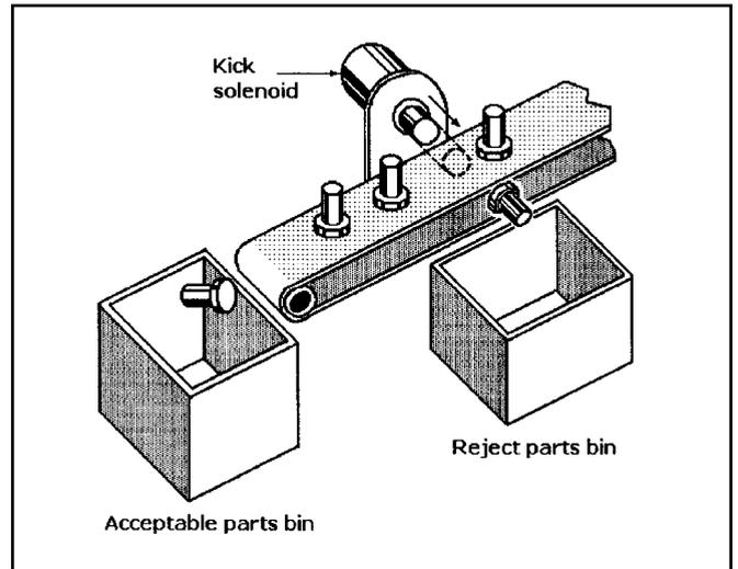
**Parts Rejection:** A push-out linear solenoid can rapidly expel or reject parts that are moving past it into a bin when triggered. An electronic video or proximity sensing system is required to energize the solenoid at the right time.
