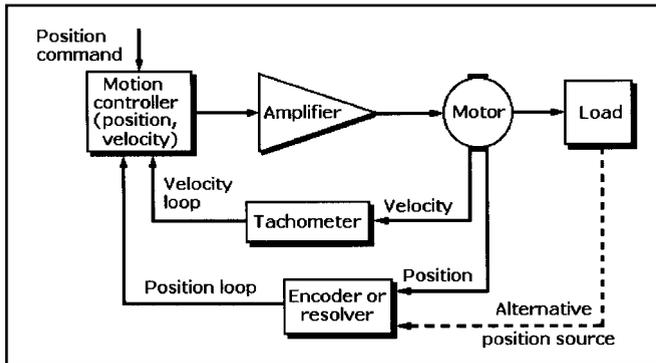
**Fig. 5** Block diagram of a position-control system.
