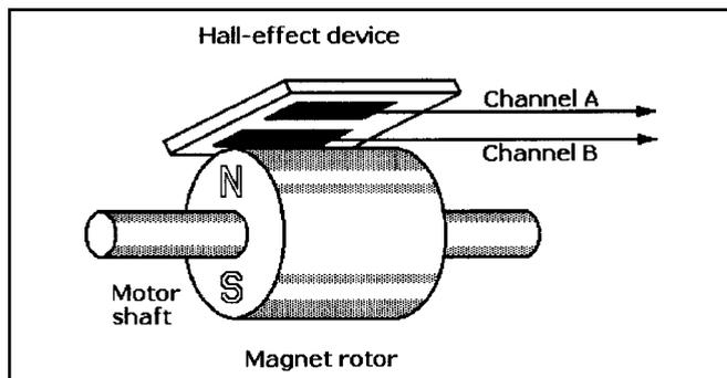
Fig. 6 Basic parts of a magnetic encoder.
