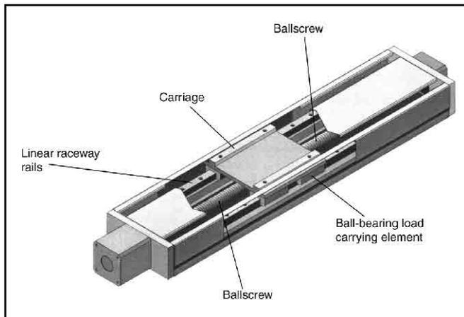
**Fig. 1** This commercial ballscrew-actuated system offers position accuracy of 0.025 mm per 300 mm with repeatability of  $\pm 0.005$  mm. Its carriage can move at speeds up to 1 m/s. It has T-slots in its base mounting system and is designed to be continuously supported. *Courtesy of Thomson Industries, Inc.*
