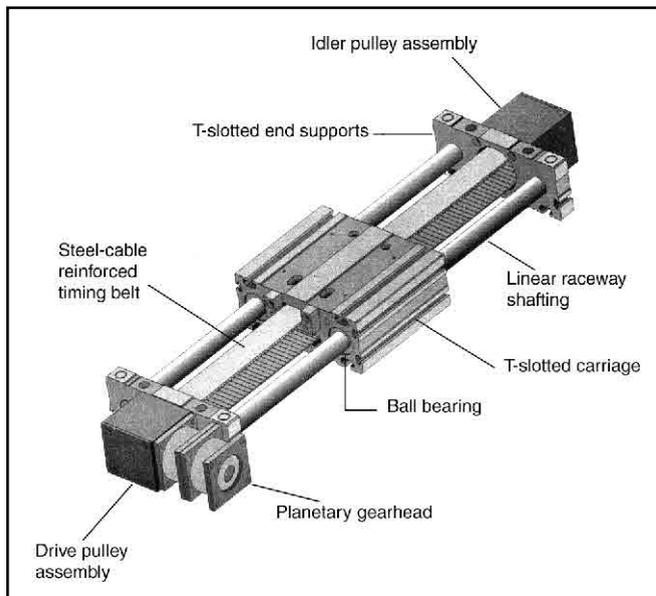
**Fig. 3** This modular single-axis belt-driven system is built to bridge a gap between its supporting surfaces. Position accuracy is better than  $\pm 0.15$  mm and speed can reach 5 m/s, both higher than for a ballscrew-driven system. A precision gearhead matches the inertia between system payload, and the servomotor provides thrust to 1400 N-m at speeds up to 4000 rpm. *Courtesy of Thomson Industries, Inc.*
