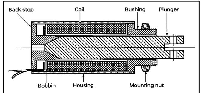
**Fig. 2** Cross-section view of a commercial linear pull-type solenoid with a clevis. The conical end of the plunger increases its efficiency. The solenoid is mounted with its threaded bushing and nut.
