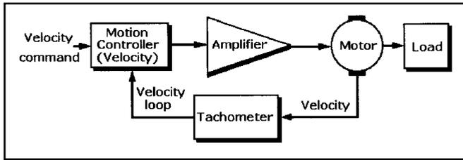
**Fig. 4** Block diagram of a velocity-control system.
