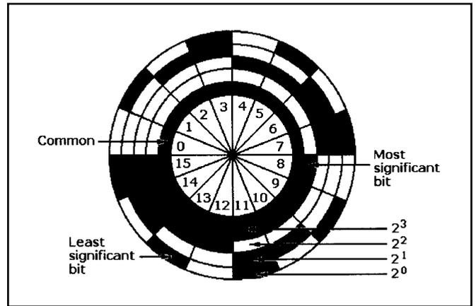
**Fig. 4** Binary-code disk for an absolute optical rotary encoder. Opaque sectors represent a binary value of 1, and the transparent sectors represent binary 0. This four-bit binary-code disk can count from 1 to 15.
