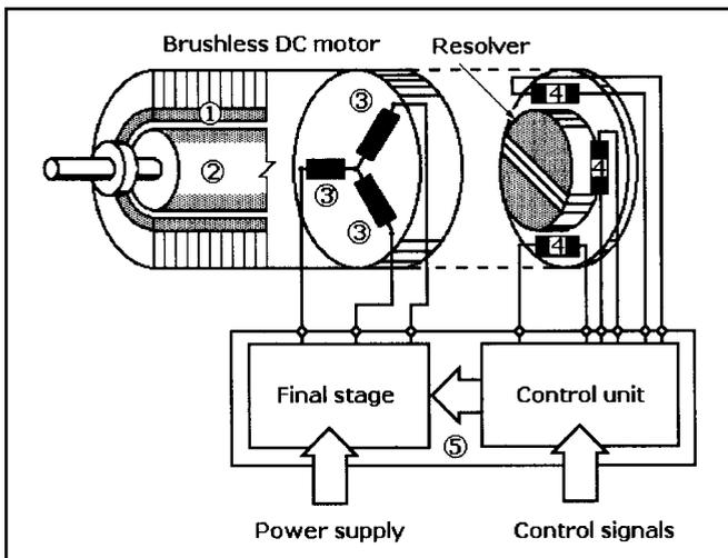
**Fig. 10** A resolver as a rotor position indicator: stationary motor winding (1), permanent-magnet motor rotor (2), three-phase electronically commutated field (3), three magnetic sensors (4), and the electronic circuit board (5).
