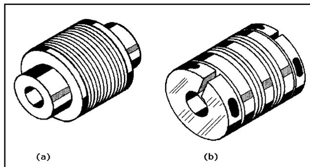
**Fig. 16** Bellows couplings (a) are acceptable for light-duty applications. Misalignments can be  $9^\circ$  angular or  $\frac{1}{4}$  in. parallel. Helical couplings (b) prevent backlash and can operate at constant velocity with misalignment and be run at high speed.
