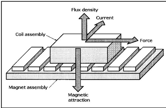
Fig. 11 Operating principles of a linear servomotor.
