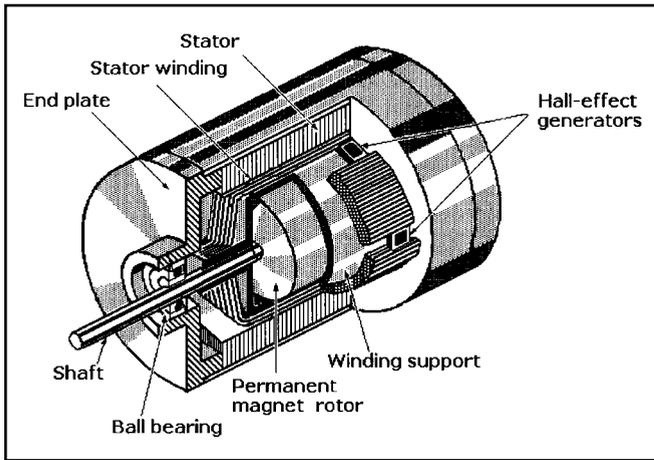
Fig. 6 Cutaway view of a brushless DC motor.
