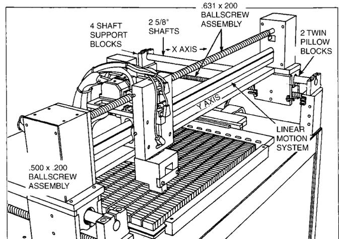
**Fig. 4** X-Y Inspection System: Catalog pillow and shaft-support blocks, ballscrew assemblies, and a preassembled motion system were used to build this system, which accurately positions an inspection probe over small electronic components. *Courtesy of Thomson Industries, Inc.*
