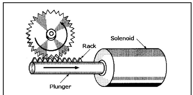
**Ratcheting Mechanism:** A pull-in solenoid with a rack mounted on its plunger becomes a ratcheting mechanism capable of turning a gear for the precise positioning of objects under operator or automated control.
