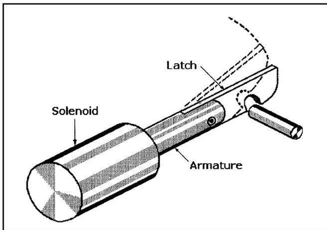
**Latching:** Linear solenoid push-out or pull-in motion can be used in a wide variety of latching applications such as locking vault doors, safe deposit boxes, secure files, computers, and machine tools, depending on how the movable latch is designed.
