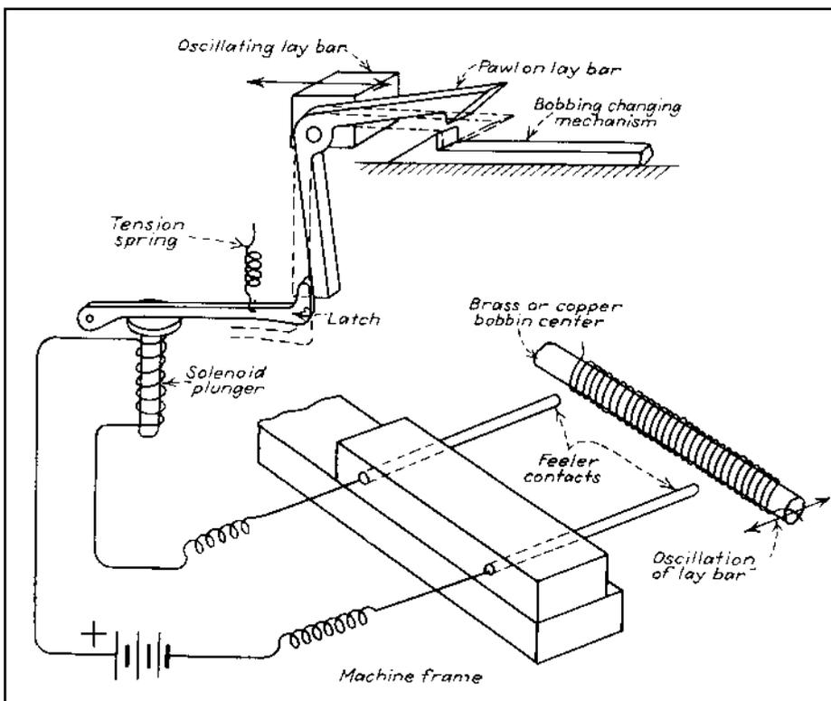
**Fig. 3** Bobbin changer. When a bobbin is empty, the feeders contact the metal bobbin center, completing the circuit through a solenoid which pulls a latch. That causes the bobbin-changing mechanism to operator and put a new bobbin in the shuttle. As long as the solenoid remains deenergized, the pawl on the lay bar is raised clear of the hook on the bobbin-changing mechanism.
