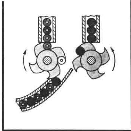
Two counter rotating wheels form a simple device for alternating the feed of two different workpieces.
