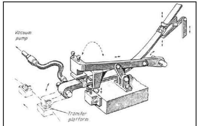
**Feeding special-shaped parts.** Parts of such special shapes as shown are removed, one by one, in a given direction, and are then moved individually into the corresponding indents on transfer platforms.
