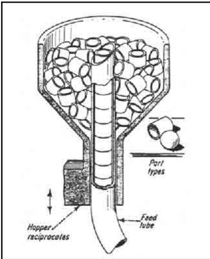
A **reciprocating feed** for spheres or short cylinders is one of the simplest feed mechanisms. Either the hopper or the tube reciprocates. The hopper must be kept topped-up with parts unless the tube can be adjusted to the parts level.
