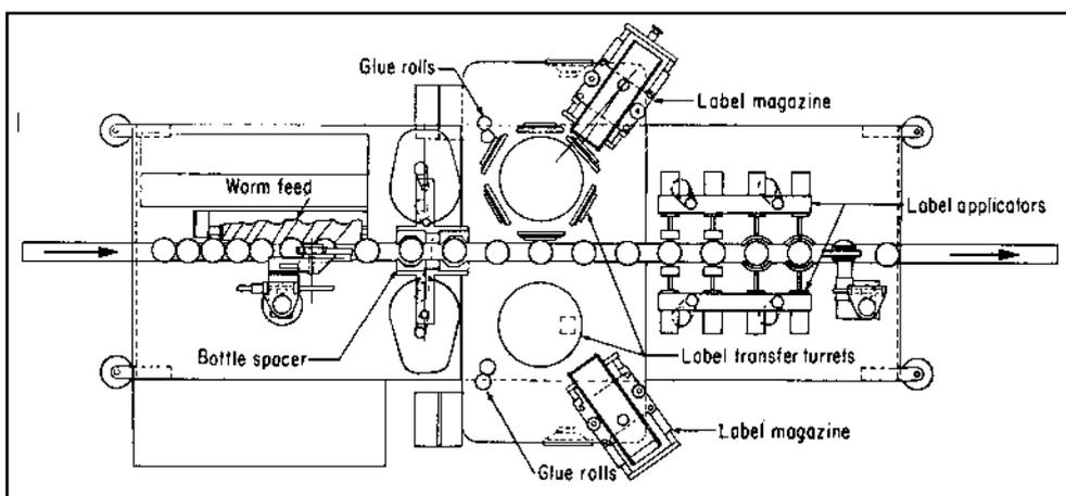
The flow of containers through this labeler is shown by the top-view drawing of the machine. Bottle spacers ensure that containers remain  $7\frac{1}{2}$  in. apart on the conveyor. Dual label-transfer turrets allow for the simultaneous application of front and back labels.
