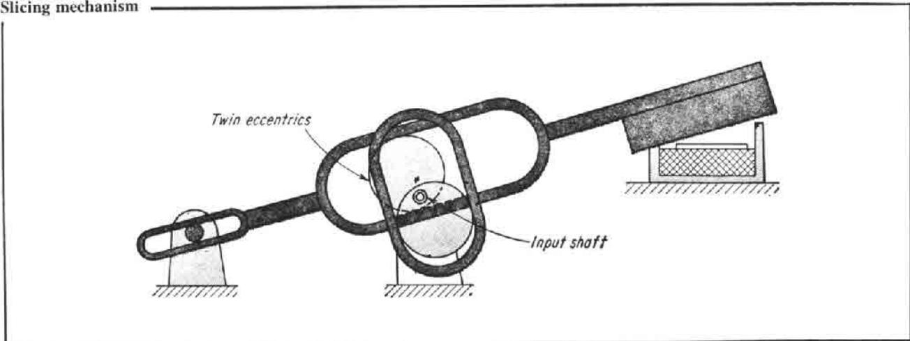
Slicing motion is obtained from the synchronized effort of two eccentric disks. The two looped rings actuated by the disks are welded together. In the position shown, the bottom
