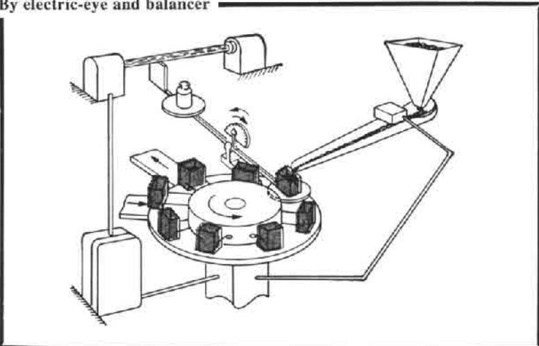
The indexing table automatically stops at the feed station. As the material drops into the container, its weight pivots the screen upward to cut off the light beam to the photocell relay. This in turn shuts the feed gate. The reactivation of the indexing table can be automatic after a time delay or by the cutoff response of the electric eye.
