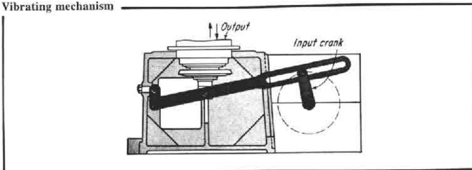
As the input crank rotates, the slotted link, which is fastened to the frame with an intermediate link, oscillates to vibrate the output table up and down.
