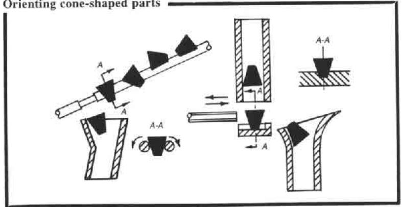
Regardless of which end of the cone faces forward as the cones slide down the cylindrical rods, the fact that both rods rotate in opposite directions causes the cones to assume the position shown in section A-A (above). When the cones reach the thinned-down section of the rods, they fall down into the chute, as illustrated.
