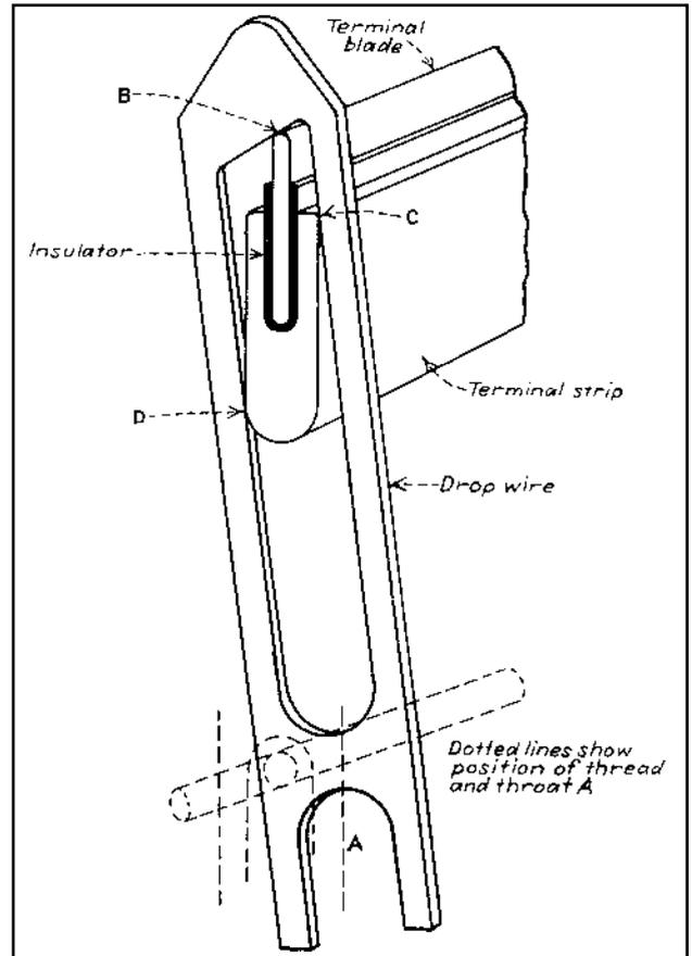
**Fig. 2** An electrical three-point wedging "warp stop" is shown after a thread has broken and a drop wire has fallen and tilted to close the circuit. Dotted lines indicate the normal position of the drop wire when it is riding on a thread. When a thread breaks, the drop wire falls and strikes the top of the terminal blade B, the inclined top of the slot. This causes a wedging action that tilts the drop wire against the terminal strip at C and D, reinforcing the circuit-closing action.
