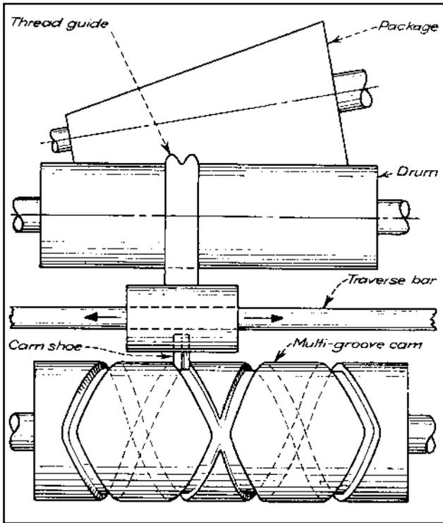
**Fig. 4** A drum drives the package by friction. A pointed cam shoe, which pivots in the bottom side of the thread guide assembly, rides in cam grooves and produces a reciprocating motion of the thread guide assembly on the traverse bar. Plastic cams have proved to be satisfactory even with fast traverse speeds. Interchangeable cams permit a wide variety of winding methods.
