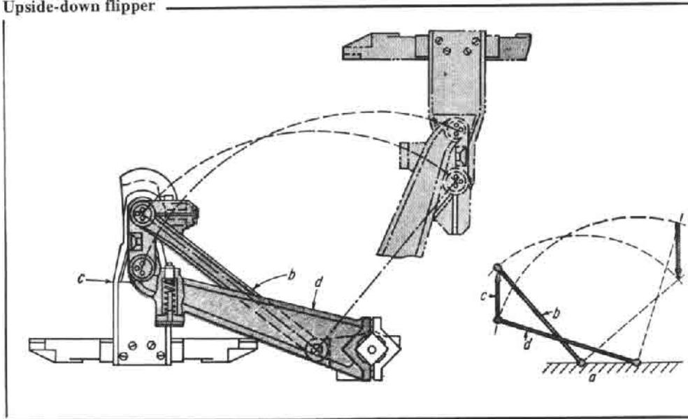
This is a four-bar linkage (links *a*, *b*, *c*, *d*) in which the part to be turned over is coupler *c* of the linkage. For the proportions shown, the 180° rotation of link *c* is accomplished during the 90° rotation of the input link.
