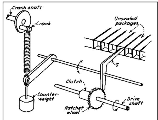
**Fig. 24** some package-loading machines have provisions to stop the machine if a package passes the loading station without receiving an insert. Pawl finger *F* has a rocking motion imparted by the crankshaft, timed so that it enters the unsealed packages and is stopped against the contents. If the box is not filled, the finger enters a long distance. The pawl end at the bottom engages and holds a ratchet wheel on the driving clutch which disengages the machine-driving shaft.
