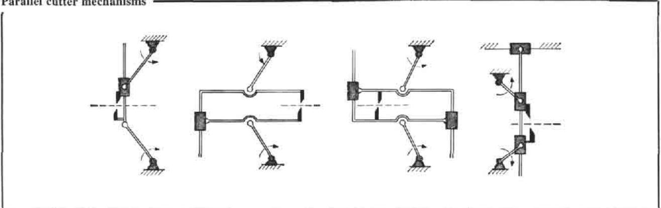
The cutting edges of the knives in the four mechanisms move parallel to each other, and they also remain vertical at all times to cut the material while it is in motion. The two cranks are rotated with constant velocity by a 1 to 1 gear system (not shown), which also feeds the material through the mechanism.
