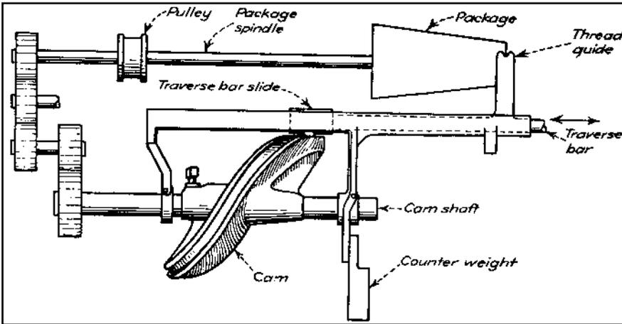
**Fig. 1** A package is mounted on a belt-driven shaft on this precision winding mechanism. A camshaft imparts reciprocating motion to a traverse bar with a cam roll that runs in a cam groove. Gears determine the speed ratio between the cam and package. A thread guide is attached to the traverse bar, and a counterweight keeps the thread guide against the package.
