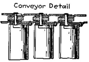
This pasteurizer carrier links lock bottles in place on straight ways.
