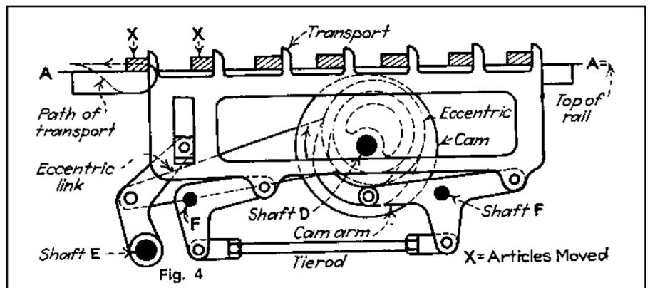
**Fig. 4** This drawing illustrates an action in which the forward motion is imparted by an eccentric while the raising and lowering of the transport is accomplished by a cam. The shafts, *F*, *E*, and *D* are positioned by the frame of the machine. Special bell cranks support the transport and are interconnected by a tierod.
