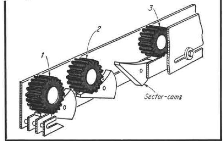
Each gear in this device is held up by a pivotable cam sector until the gear ahead of it moves forward. Thus, gear 3, rolling down the chute, kicks down its sector cam but is held up by the previous cam. When gear 1 is picked off (either manually, or mechanically), its sector cam pivots clockwise because of its own weight. This permits gear 2 to move into place of gear 1—and frees cam 2 to pivot clockwise. Thus, all gears in the row move forward one station.
