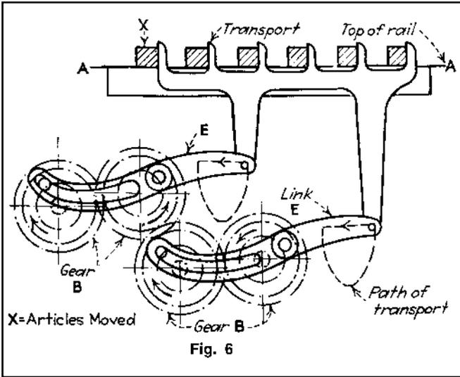
**Fig. 6** An arrangement of interconnected gears with equal diameters that will impart a transport motion to a mechanism. The gear and link mechanism imparts both the forward motion and the raising and lowering motions. The gear shafts are supported in the frame of the machine.
