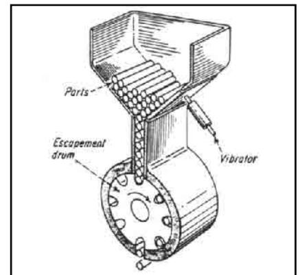
A **long-cylinder feeder** is a variation of the first two hoppers. If the cylinders have similar ends, the parts can be fed without proposition, thus assisting automatic assembly. A cylinder with differently shaped ends requires extra machinery to orientate the part before it can be assembled.
