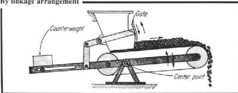
The loose material falls down the hopper and is fed to the right by the conveyor system which can pivot about the center point. The frame of the conveyor system also actuates the hopper gate so that if the amount of material on the belt exceeds the required amount, the conveyor pivots clockwise and closes the gate. The position of the counterweight on a frame determines the feed rate of the system.
