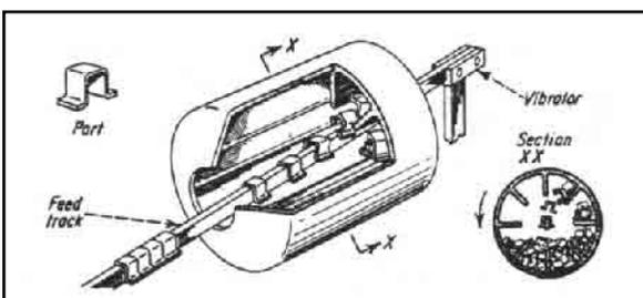
A **barrel hopper** is useful if parts tend to become entangled. The parts drop free of the rotating-barrel sides. By chance selection, some of them fall onto the vibrating rack and are fed out of the barrel. The parts should be stiff enough to resist excessive bending because the tumbling action can subject them to relatively severe loads. The tumbling can help to remove sharp burrs.
