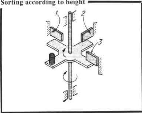
Workpieces of varying heights are placed on this slowly rotating cross-platform. Bars 1, 2, and 3 have been set at decreasing heights beginning with the highest bar (bar 1), down to the lowest bar (bar 3). The workpiece is therefore knocked off the platform at either station 1, 2, or 3, depending on its height.
