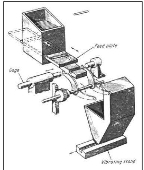
**Horizontal feed for fixed-length rods.** Single rods of a given length are brought from the hopper to the slot of a fixed plate by a moving plate. After being gauged in the notched portion of the fixed plate, each rod is moved to the chute by means of a lever, and is removed from the chute by a vibrating table.
