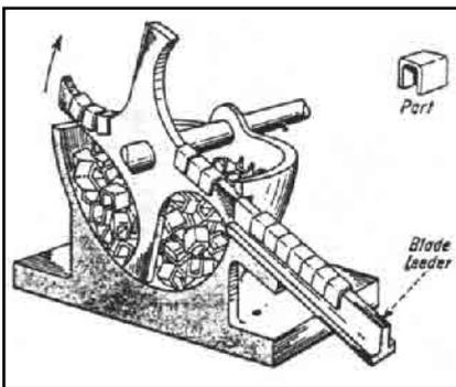
**Rotary centerblades** catch small U-shaped parts effectively if their legs are not too long. The parts must also be resilient enough to resist permanent set from displacement forces as the blades cut through a pile of parts. The feed is usually continuous.
