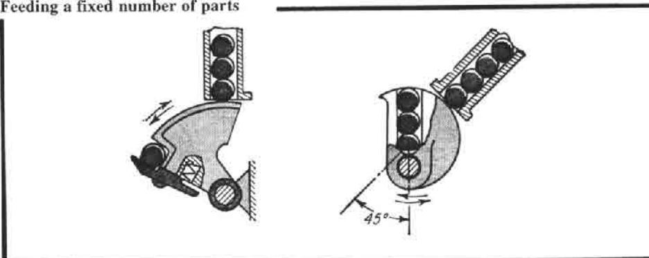
The oscillating sector picks up the desired number of parts, left diagram, and feeds them by pivoting the required number of degrees. The device for oscillating the sector must be able to produce dwells at both ends of the stroke to allow sufficient time for the parts to fall in and out of the sector.
