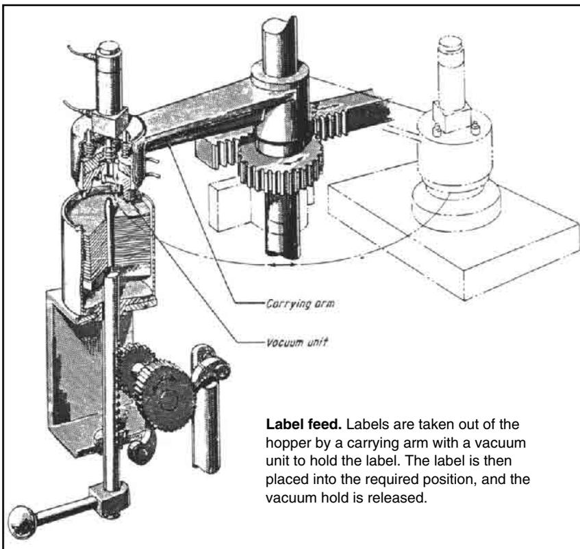
**Label feed.** Labels are taken out of the hopper by a carrying arm with a vacuum unit to hold the label. The label is then placed into the required position, and the vacuum hold is released.
