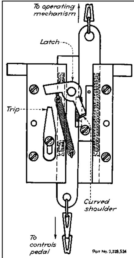
**Fig. 1** A repetition of the machine cycle is prevented if a pedal remains depressed. The latch carried by the left slide pushes the right slide downward with a curved shoulder until the latch is disengaged by trip member.
