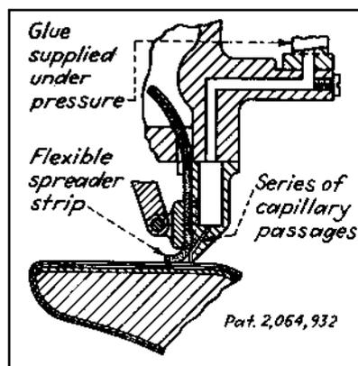
Fig. 17 Glue is extruded through nozzle on work.
