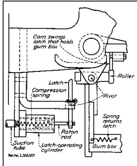
**Fig. 2** The gumming of the suction picker and label carrier when the label is not picked up by the suction is prevented by insufficient suction on a latch-operating cylinder, caused by open suction holes on the picker. When a latch-operating cylinder does not operate, the gum box holding latch returns to its holding position after cyclic removal by the cam and roller, thus preventing the gum box and rolls from rocking to make contact with the picker face.
