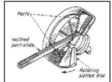
A **rotary screw-feed** handles screws, headed pins, shouldered shafts, and similar parts in most hopper feeds, random selection of chance-oriented parts calls for additional machinery if the parts must be fed in only one specific position. Here, however, all screws are fed in the same orientation (except for slot position) without separate machinery.
