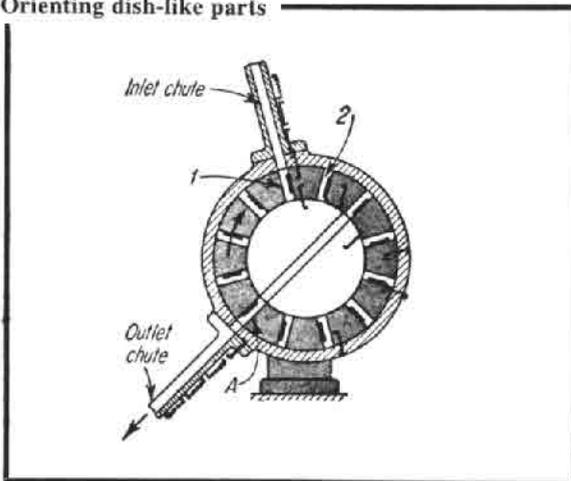
A part with its open-end facing to the right (part 1) falls on a matching projection as the indexing wheel begins to rotate clockwise. The projection retains the part for  $230^\circ$  to point A where it falls away from the projection to slide down the outlet chute, open-end up. An incoming part facing the other way (2) is not retained by the projection, hence it slides *through* the indexing wheel so that it too, passes through the outlet with its open-end up.
