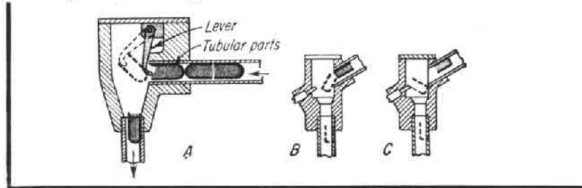
Here's a common problem; Parts arrive in either open-end or closed-end first; you need a device that will orient all the parts so they feed out facing the same way. In Fig. A, when a part comes in open-end first, it is pivoted by the swinging lever so that the open end is up. When it comes in closed-end first, the part brushes away the lever to flip over headfirst. Fig. B and C show a simpler arrangement with pin in place of lever.
