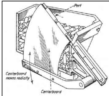
A **centerboard selector** is similar to reciprocating feed. The centerboard top can be milled to various section shapes to pick up moderately complex parts. It works best, however, with cylinders that are too long to be led with the reciprocating hopper. The feed can be continuous or as required.
