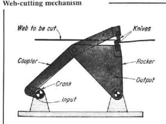
This four-bar linkage with an extended coupler can cut a web on the run at high speeds. The four-bar linkage shown is dimensioned to give the knife a velocity during the cutting operation that is equal to the linear velocity of the web.
