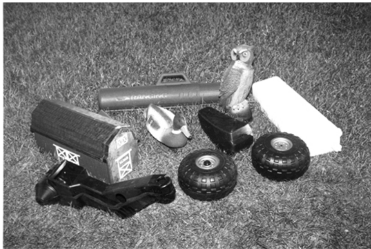
Figure 3.4 Examples of objects made using cast aluminium moulds
