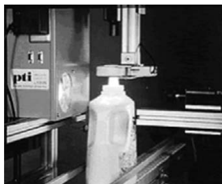
Figure 9.2 Scanning bottlenecks for defects related to thread profile, neck slant, flash, and neck diameter and height
