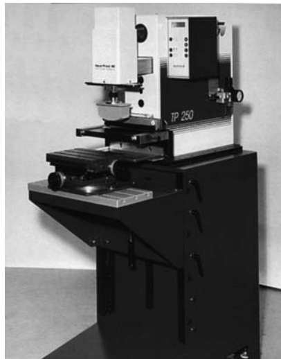
Figure 11.9 Pad printing press with inked rubber pad ready to pad print on object (football)
