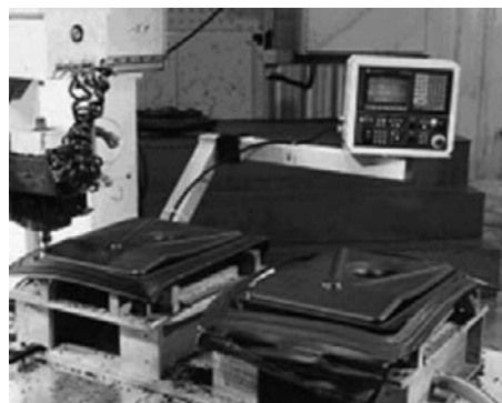
Figure 10.4 Using a CNC router to automatically trim blow moulded panels Reproduced with permission from Agri-Industrial Plastics, Fairfield, IA, USA.
