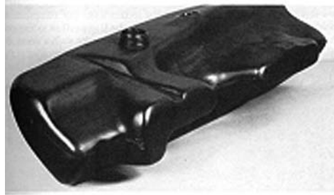
Figure 1.10 Fuel tank with layered wall
