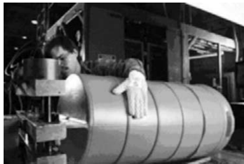
Figure 10.1 Finishing an extrusion blow moulded traffic safety barrel Reproduced with permission from Crocker Limited, Three Rivers, MI, USA.
